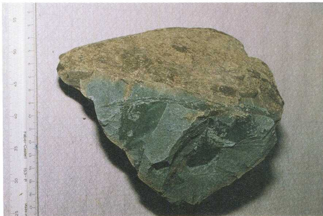
Fig 15-1. A piece of Bavarian bentonite clay (Moosburg) where oxidation has formed a redox front.
